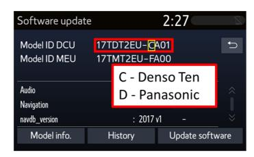
5. In the "Software update" menu: the current installed software is displayed. The DCU software is listed under "Audio".
