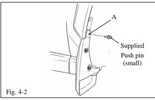
(b) Install supplied push pin (small) in location A while holding part up and into body panel (Fig. 4-2).
